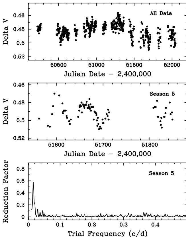
FIG. 2.—*Top*, 557 variable minus comparison differential magnitudes of HD 161570 acquired with the 0.4 m APT; *middle*,  $V$  photometry from the fifth observing season plotted on an expanded abscissa; *bottom*, frequency spectrum of the  $V$  photometry from season 5, revealing the  $64.1 \pm 0.1$  day rotation period.
