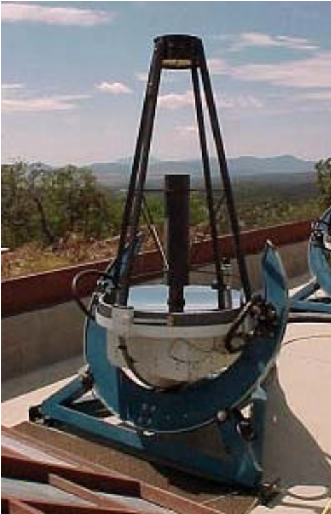
Figure 1. A modern automatic photometric telescope (T12) at Fairborn Observatory. This telescope is simple in design; it has no provisions for manual operation, although it does incorporate electronic cameras and apertures useful for periodically aligning it from the control room. It has a photometer that can be pulled out as a unit for maintenance and simple stepper drives adequate for finding and tracking stars reliably. Over the past 15 years, our APT's have collected over 400,000 group observations (a basic set of measurements of a group of three or four program and comparison stars) of the brightness of variable stars.
