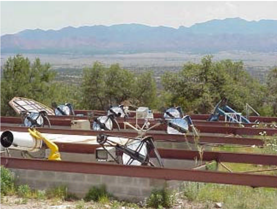
Figure 2. Seven of the twelve 0.25 to 0.80-m automatic telescopes at Fairborn Observatory in southern Arizona. The TSU 2.0-m spectroscopic telescope is located behind the camera.
