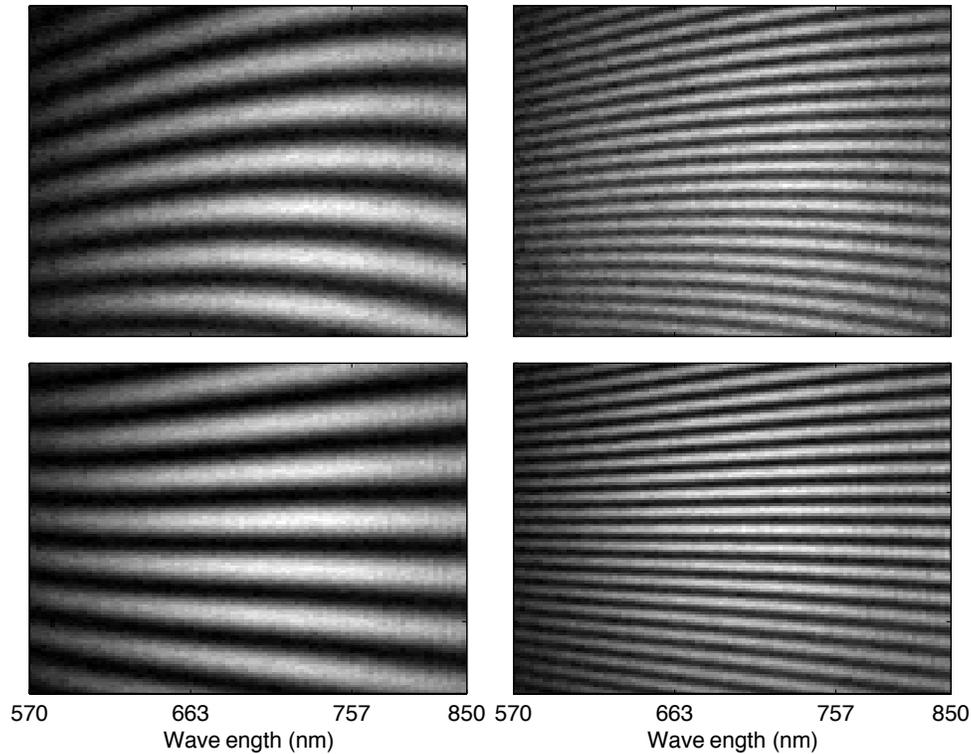
Figure 3. White light channeled spectrum produced by VISION for two different pairs with spatial frequencies of  $7f_0$  and  $18f_0$ . The horizontal axis is the spectral direction. Top: Fibers were cut with equal length. Bottom: Differential dispersions were minimized.
