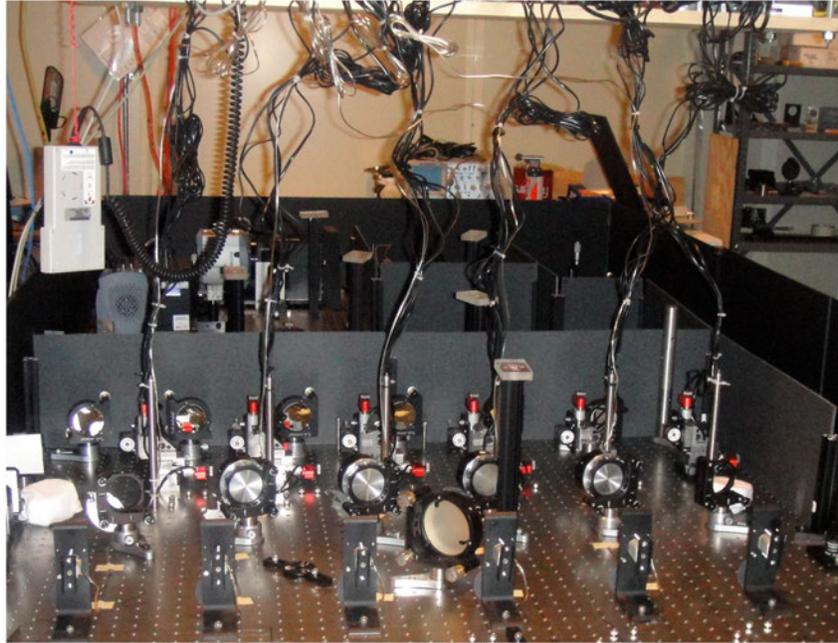
Figure 4. Fiber feed units of VISION deployed at NOI.
