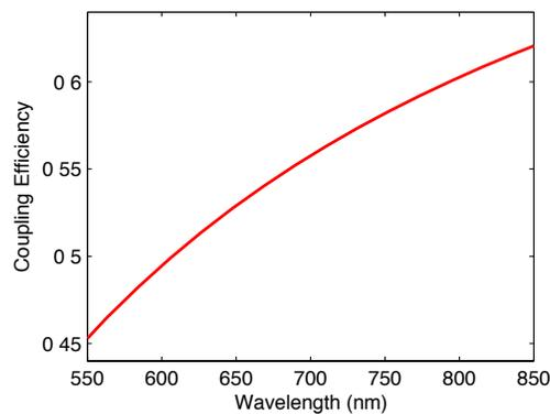
Figure 2. Theoretical coupling efficiency of the fiber feed unit with f/4.7.
