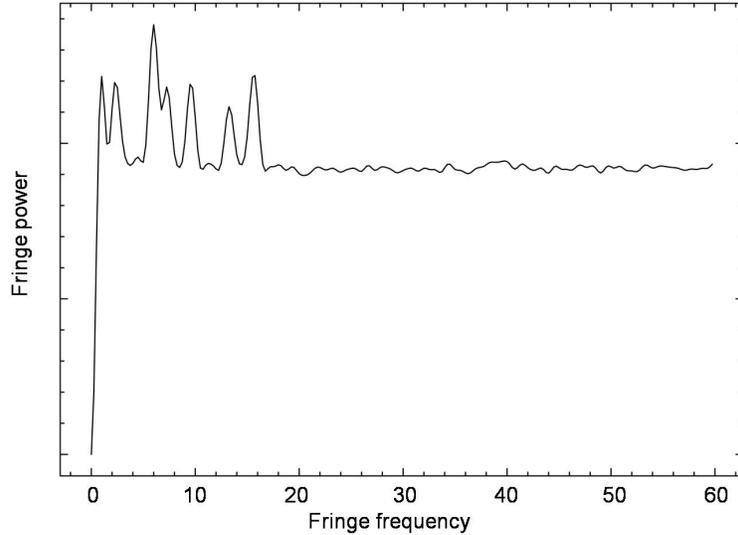
Figure 2. Fringe power spectrum in VISION data from four-element observations of an unresolved star. Units on the axes are arbitrary. The peak at fringe frequency = 1 is an artifact from the removal of the zero-frequency (total flux) signal. Six simultaneous fringe signals are seen.
