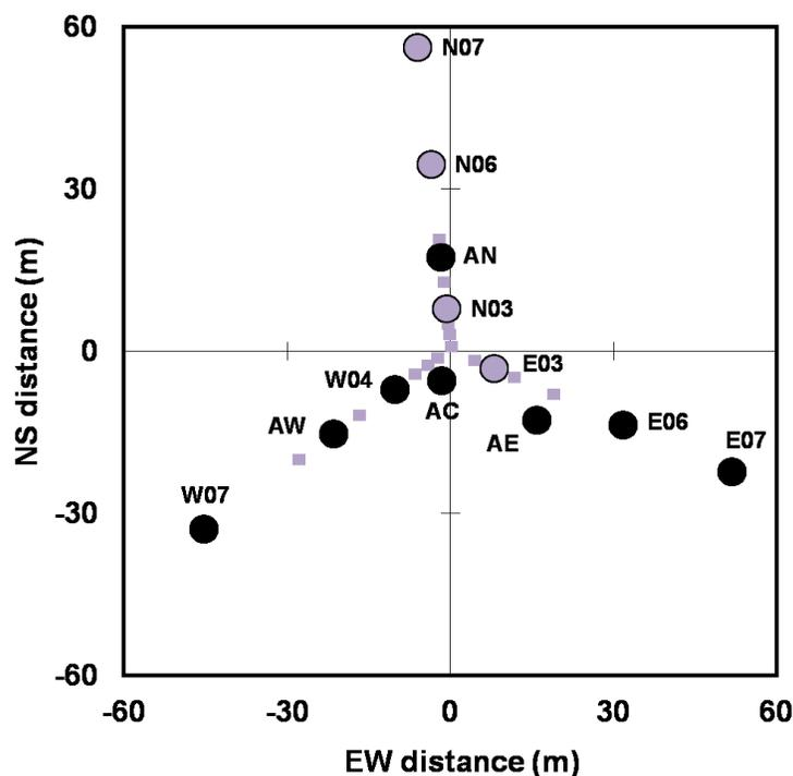
Figure 1. Available stations after current upgrades. Filled black circles indicate the stations available as of mid-2013 plus those stations that have been brought into operation recently (E07, W04). Filled gray circles indicate stations that are currently being added. The small gray squares are station locations not yet in use. Stations E10 and W10 are also nearing operational status, but at 250 m from the center of the array are beyond the borders of the figure.
